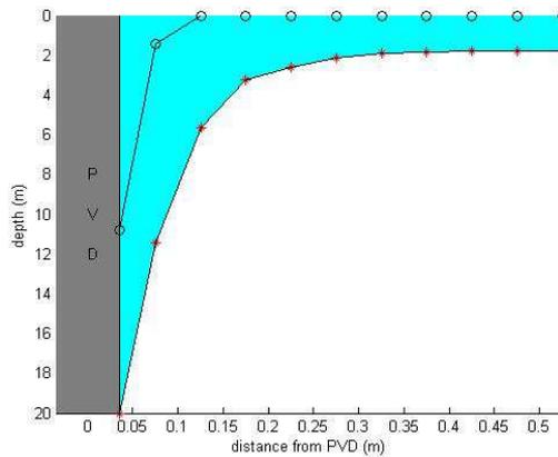
Fig. 2. Change of the effective range with consolidation time
